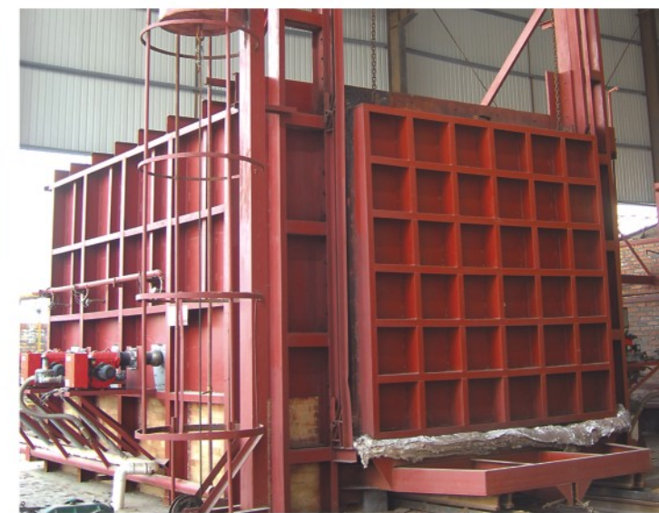
热处理炉 Heat treatment furnace
