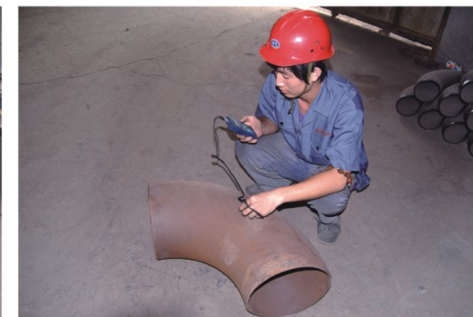
测厚 Thickness measurement
